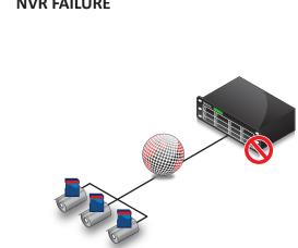
Edge Recording will take place if either the network or NVR fails. In both cases- the IP-camera will automatically take over recording and store the video-data on the onboard SD-card. In this case video-loss will be prevented. As soon the network or NVR is restored- the video-data on the SD-card will automatically be reclaimed by the NVR.
