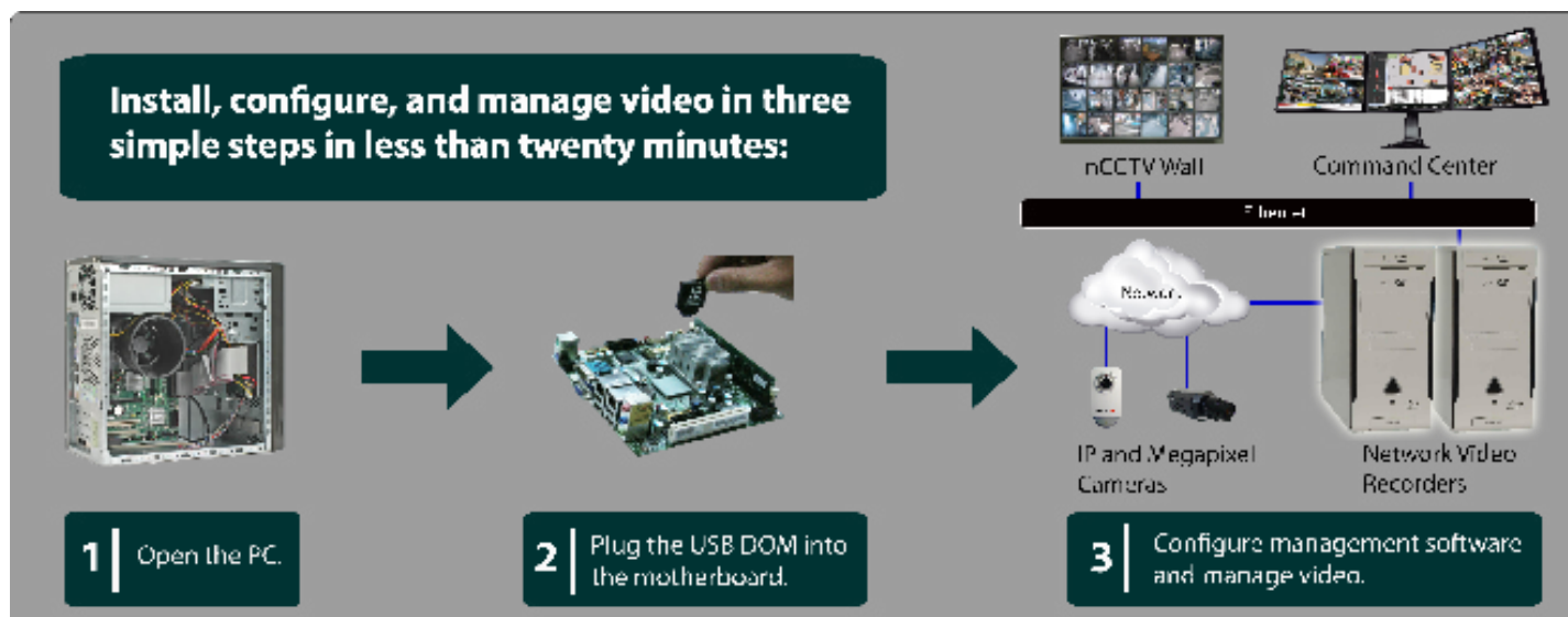
Figure 1.1 USB DOM Installation Steps (1) Open a PC that follows the NVR hardware requirements and access the motherboard. (2) Plug the USB DOM into the motherboard and close the PC. (3) Connect the PC to the surveillance system. Configure the NVR and you will be able to record and manage video on a reliable NVR using many standard PC parts.
